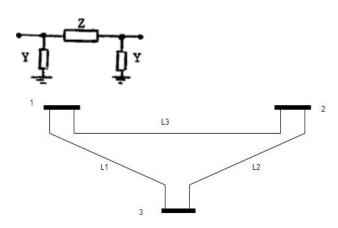
To simplify consider that Y and Z have the same value for each line. Assume also that each node has an injected complex power given by:
