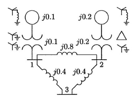
Each generator is represented by an emf behind the transient reactance. All impedances are expressed in per unit on a common 100 MVA base, and for simplicity, resistances are neglected. The following assumptions are made.
