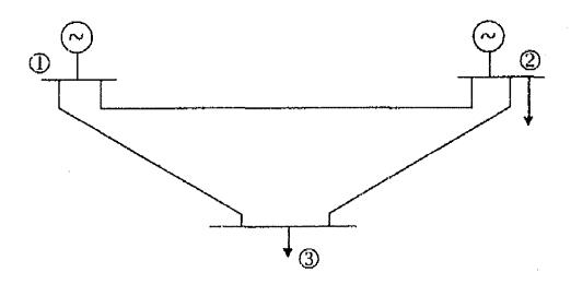
Choose Bus 1 as the reference bus, and, for simplicity, assume that the lines have all the same series impedance  $Z_s$  and the admittance  $Y_p/2$  in the  $\pi$ - model of the line.
