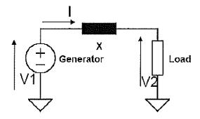
This figure shows a generator connected to a load through a reactance, which includes both the generator and line reactances. The real power transmitted by the generator and the reactive power supplied to the load, assuming a constant voltage V<sub>2</sub>, are given by the following formulas:
