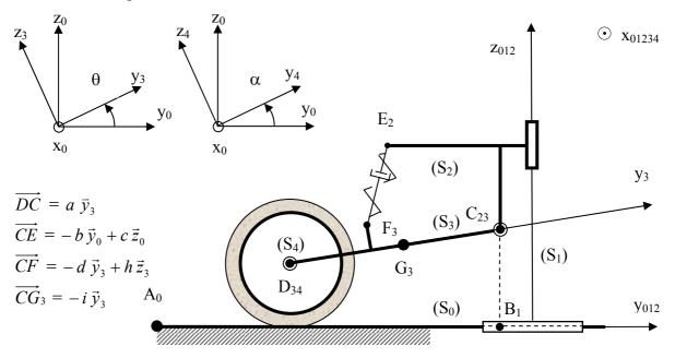
The rear part of the framework of the scooter, loaded with the corresponding mass of the driver, is assumed to be moving in translation with respect to the road. This assumption is represented in the form of an additional intermediate body  $(S_1)$ , of negligible mass located between the road  $(S_0)$  and the framework of the scooter  $(S_2)$  by means of two prismatic joints.
